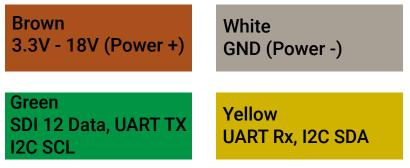
**Output signal**: SDI-12 version1.4; address factory set to 0 (default) , Uart (configurable), I2c (configurable)
