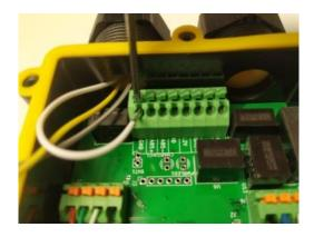
4. Tighten the holder in order to fix the cable and close the gateway with the screws. (To achieve the IP68 rating, all glands must be occupied by round-section cables of between 4.5mm and 10mm or be replaced by blanking plugs)
