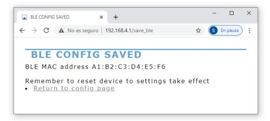
In the case no MAC is configured, the NMEA Connect Plus will connect the first ULTRASONIC BLE device detected.
