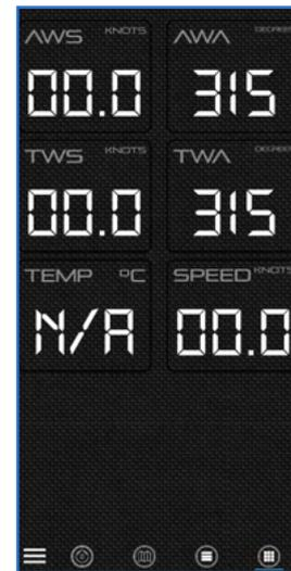
At the bottom of the main menu, there are four screen options you can choose from: main screen, wind line graph, wind bar graph, and multiple data.
