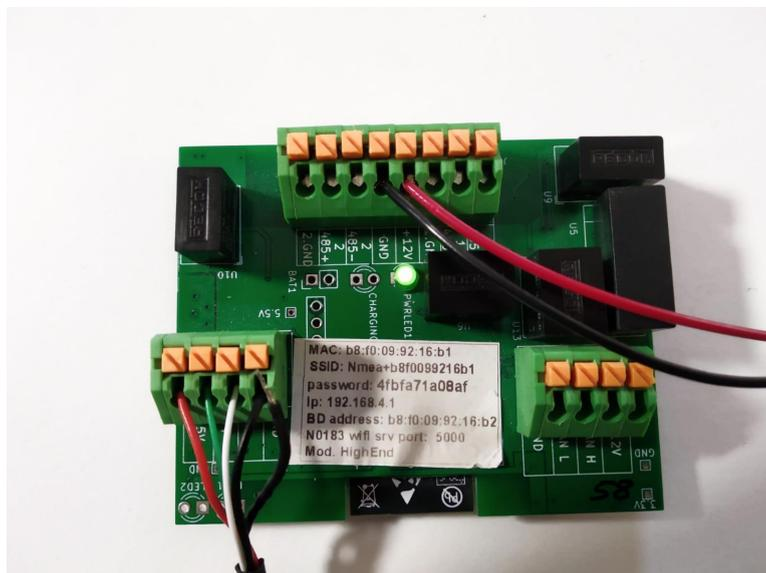
2. We connect the cables of our display or chart plotter to Port 2 of the top terminal. The **0183 input** cable goes to **2.485+**. The **0183 output** cable goes to **2.485-**. It is important to make a **bridge** that connects **2.GND** (where we have the ground wire of the display connected) to **GND** (where we have the ground wire connected from the energy source) as indicated with the yellow arrows. Connect the **display's power** to
